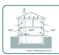
Some studies suggest that the un-insulated air-leaky basement can be responsible for 30% or more of a home's heat loss. Air-seal the basement for sure! But you can also insulate the basement walls with one of the new fire-rated foams. If you have sufficient height in your ceiling, a new cellar slab over rigid foam insulation can be installed with great results. Wright Builders does this work with talented, resourceful trade's people and the best materials.
